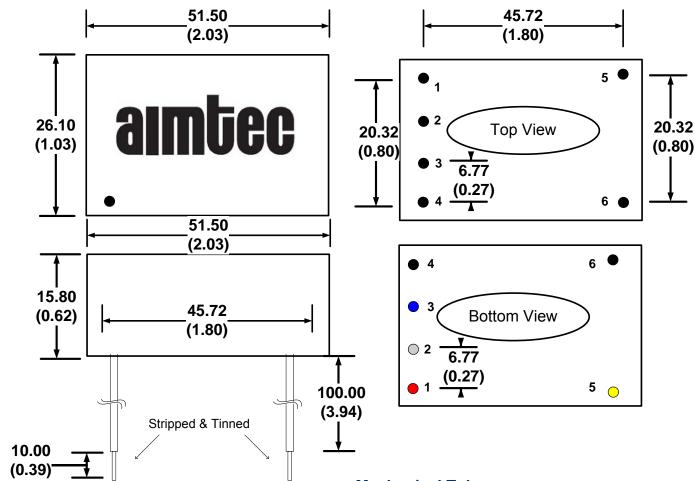
\*Lead Wires are under the specifications of general lamps: \*Wire is UL 1015/CSATEM listed #22AWG / 600V / 105°C
