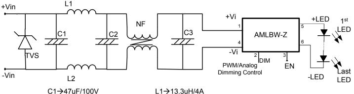
C1→47uF/100V C2→330uF/100V C3→330uF/100V TVS→38V
