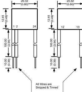
Lead Wires are under the specifications of general lamps Wire is UL 1015/CSATEM listed #22AWG / 600V / 105°C
