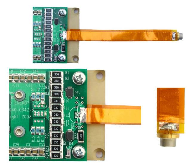
Figure 11 – Diode / Driver Interconnection Using DEI 1820-0030 Stripline Material
