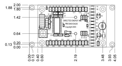
Figure 2B – PCO-7120 Dimensional Drawing With Heat Spreader
