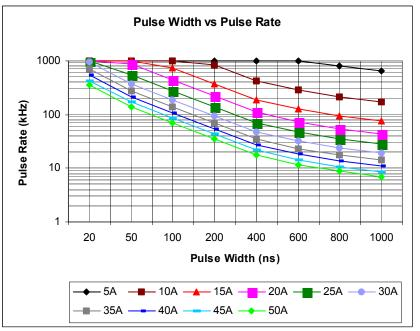
Figure 1 – Maximum Pulse Width vs Maximum Frequency
