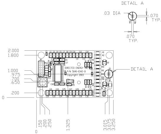
Figure 2A – PCO-7120 Dimensional Drawing – Circuit Board Only
