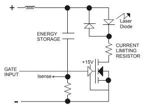
gate drive circuit. This design provides a high degree of reliability, excellent switching performance, variable pulse width and superior amplitude and temporal stability over a broad operating temperature range.
