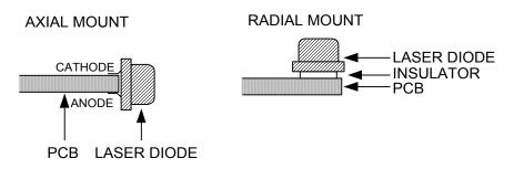
Figure 7 - Axial and Radial Mounting Positions
