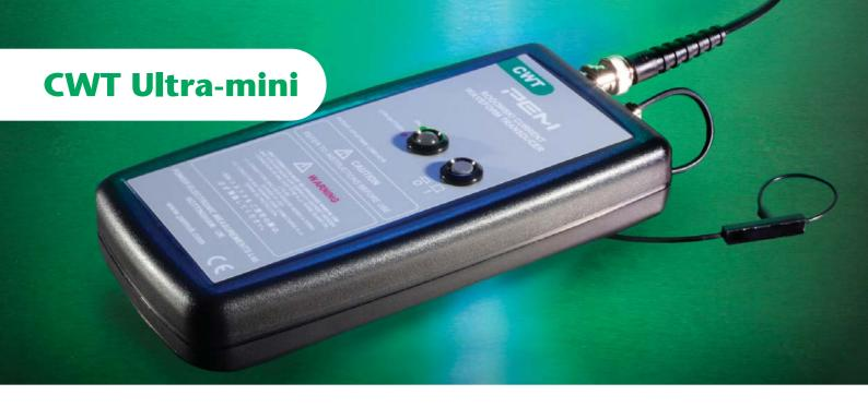
The CWT Ultra-mini has an extremely thin, clip-around Rogowski coil of typically 1.6mm cross-section. Such a thin coil enables currents to be measured in the most difficult to reach parts of a power electronic converter with negligible disruption to the circuit under test.
