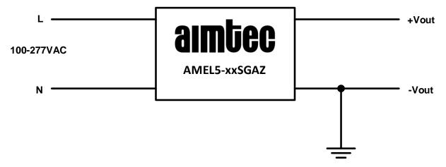
AMEL5-xxSGAZ models meet the EN55022 class B compliance when connected to Earth/Ground. These models are incorporating an EMC compliant filter and when connected to Earth/GND, no external filtering will be needed to meet the specified limits.
