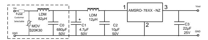
NOTE: This part is not designed for parallel operation
