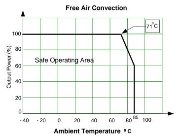
NOTE: With air convection speed of 0.8m/sec
