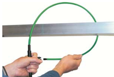
Clip the probe around the dc busbar
