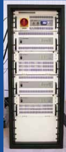
BT10K-Alpha amplifier 104.95MHz, 10kW CW Institute for Storage Ring Facilities, Aarhus University, Denmark
