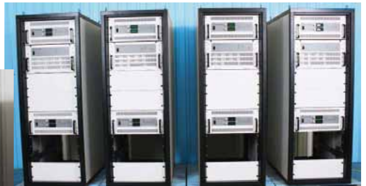
8 independent BT4K-Alpha amplifiers - 72.75MHz, 4kW CW 100% power reflection handling Produced in 2 stages: stage 1 8x2kW amplifiers (shown in photo), stage 2 upgrade to 8 x 4kW
